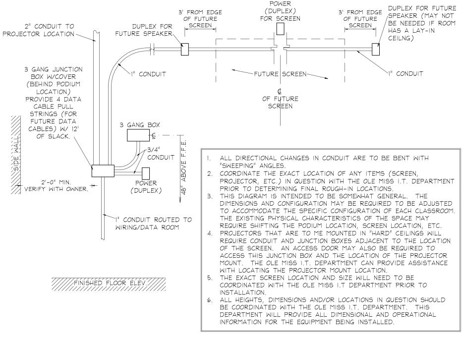
CONFIGURATION OF CONDUIT, JUNCTIONS BOXES, ETC. IN WALLS FOR FUTURE TECHNOLOGY TO BE INSTALLED IN "SMART CLASSROOMS"
